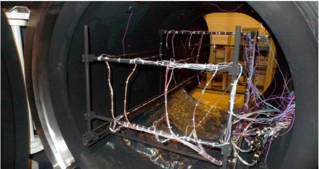
Fig. 1. Single wire batch located in the Harness Derating Test Facility at NLR
